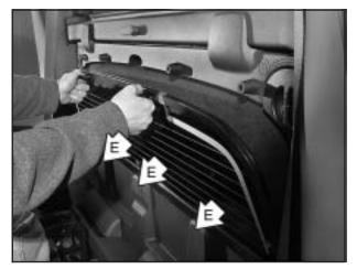
Load the rear glass into the storage pocket in the midgate, guiding the lower edge of the rear glass behind the three rear glass retaining tabs (E).
